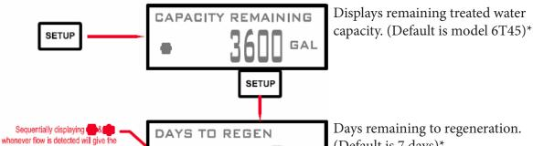
(Default is 7 days)\* appearance of a meter turbine rotating. SETUP Displays contact name and phone XXXXXXXXXXXXXXX number (if programmed)
